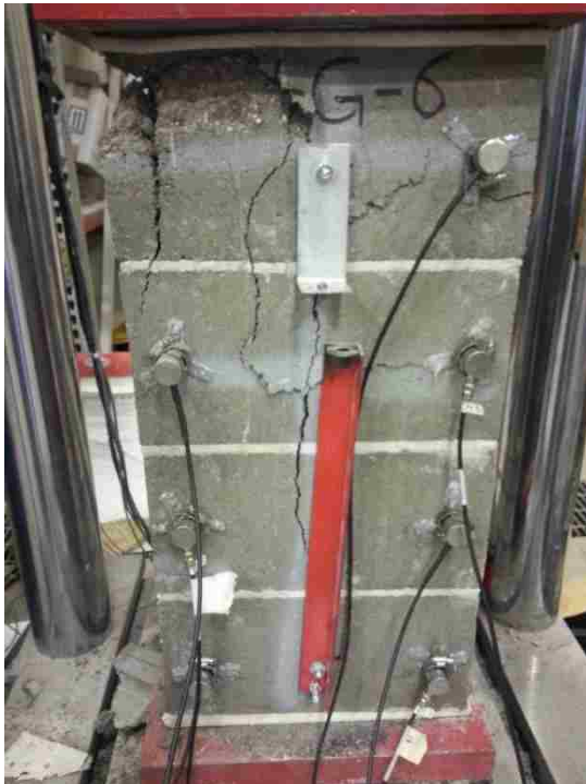
(c) 37% Rubber CMU Grouted
