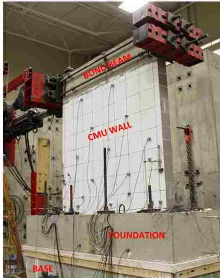
Figure 4.1. Masonry shear wall setup showing components
