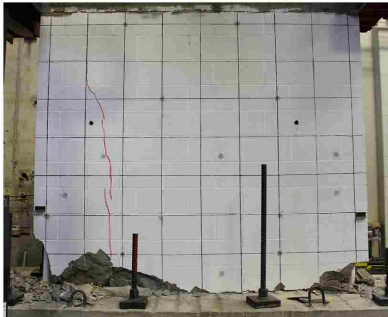
Figure 4.10. Shear Wall Two damage (vertical shear crack shown in red)
